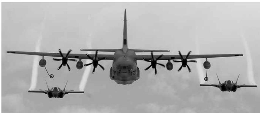
**Figure 10. KC-130 with two F-35B Lightning II Joint Strike Fighters.** This Marine Corps KC-130 also is capable of operating from Tier 3 airstrips and conducting air refueling operations.
