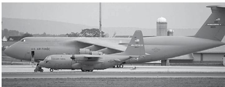
**Figure 5. C-130 (foreground) parked next to C-5.** A single photo illustrates the global-theater air cargo compatibility gap.
