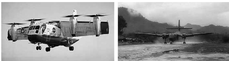
**Figure 4. XC-142A and C-7.** *left:* XC-142A being tested by NASA in 1969. This aircraft could take off and land vertically or on airstrips just a few hundred feet long with heavier loads. (Photograph courtesy of NASA, [https://crgis.ndc.nasa.gov/historic/LTV\\_XC-142A](https://crgis.ndc.nasa.gov/historic/LTV_XC-142A)); *right:* C-7 Caribou operating from a Tier 3 airstrip during the Vietnam War.
